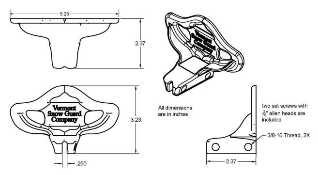
Model SS1 is made to be used with standing seam roof installations. It is suitable for seams 1 ½" or less, 24 gauge or lighter metal, and can be used on double-locked seams or seams that have been crimped over at installation point by a professional installer/roofer. (See drawing at right)
